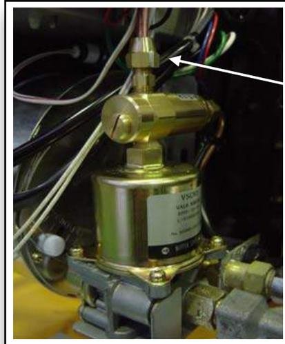
Loosen the brass nut, then check whether fuel comes out (The switch must be turned ON)
