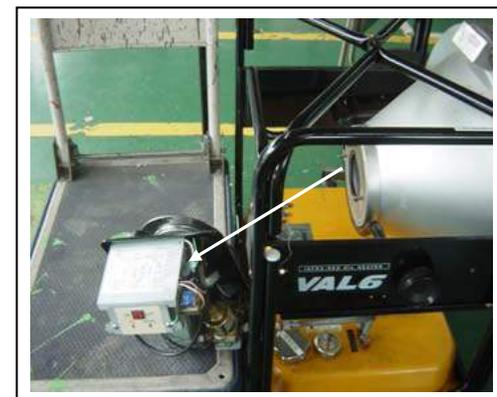
**Picture 4 Inspection of the fuel pump**
