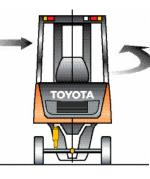
When it senses instability, SAS instantly engages the **Swing Lock Cylinder** to stabilize the rear axle, creating the lateral stability needed to help reduce the risk of lateral tipovers.
