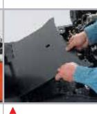
**No-tool floorboard** lifts out in seconds for fast, easy access during daily operator checks.
