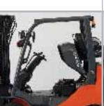
**Easy-lift engine hood** features a convenient, wideaccess design and an assist damper that automatically holds the hood open at 75 degrees for easier access to the engine compartment.
