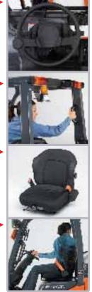
Fully hydraulic power steering system provides smooth, responsive operation while isolating vibration and shock from the operator's hands, helping reduce operator fatigue.
