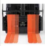
Optional integral sideshifter minimizes truck movements for storing and retrieving loads—to increase overall operator efficiency.
