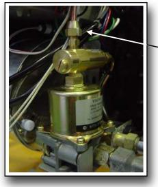
Loosen the brass nut, then check whether fuel comes out (The switch must be turned ON) If fuel is not flowing a minmum of 2" review the " How to restore the fuel flow" on page 33.
