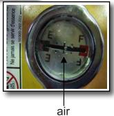
If air intake of fuel gauge is clogged, clean it
