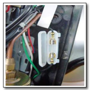
Open the fuse box and check the fuse
