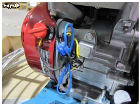
Step 14: Wrap and secure engine safety shut-off wire. (Fig. 18)
