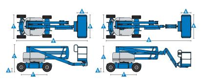
\* The metric equivalent of working height adds 2 m to platform height. U.S. adds 6 ft to platform height. \*\* In lift mode (platform raised), the machine is designed to operate on firm, level surfaces only.
